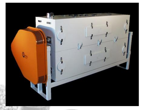
Our agitators are complete with class IIG/ID explosion proof motors, drives, and guards. All of this will be mounted on a compact sanitary square steel frame. Our standard agitators have one chlorine inlet per log with a 304 Stainless Steel flour inlet and a 304 Stainless Steel flour outlet. On both sides we will have an inspection door and two clean out doors, one at the inlet and one at the discharge.
